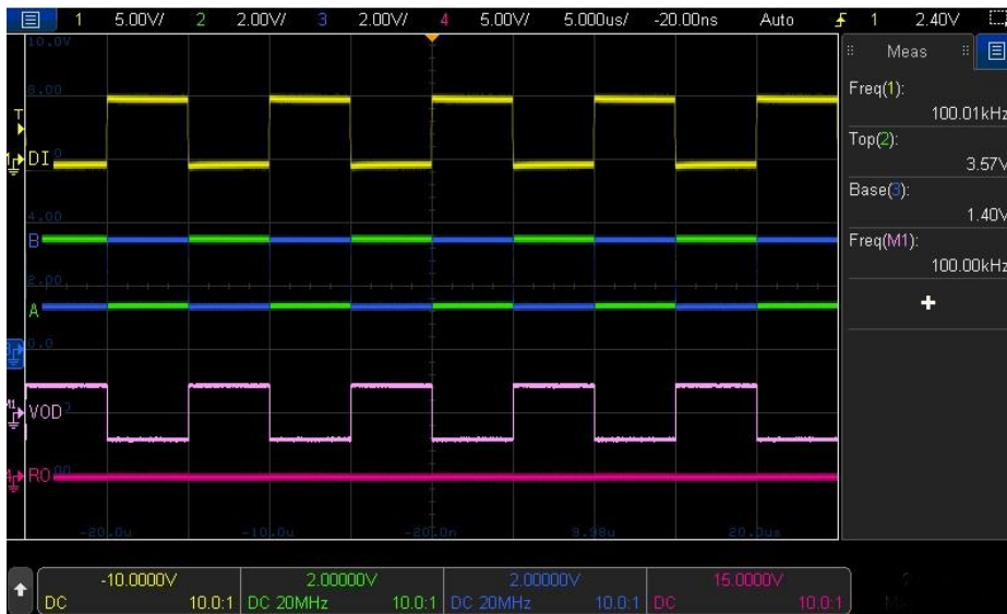
200Kbps waveform of Driver mode ( \overline{RE}=V_{CC} , DE=V_{CC} )
