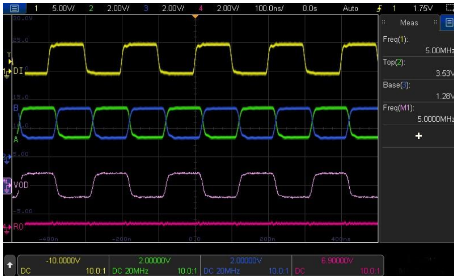
10Mbps waveform of Driver mode ( \overline{RE}=V_{CC} , DE=V_{CC} )
