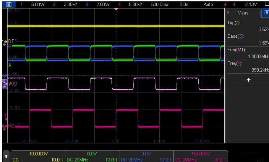
2Mbps waveform of Receiver mode ( \overline{RE} = GND , DE = GND )
